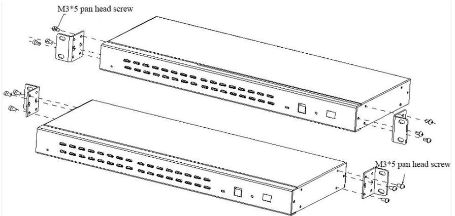
3) Screw the KVM device to the rack cabinet(front or rear part)
