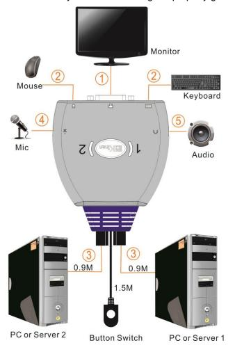
DVI Devices connected to ①: Monitor, projector
